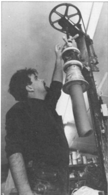
Sherrill's extruder is inverted and rotates to allow expedient production, consistent wall thickness and easier manipulation of each piece.
